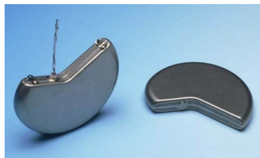
Fig. 1 Laser beam welding of titanium pacemaker cases provides a smooth, low heat input, hermetically acceptable and reliably producible weld joint [8]
