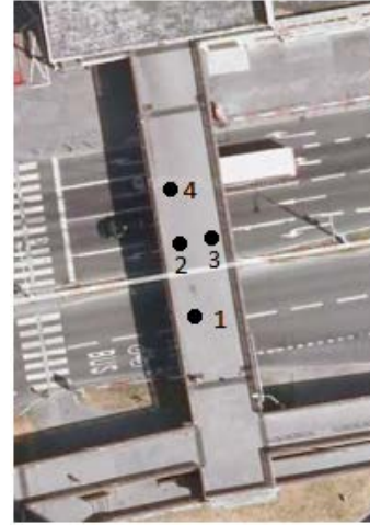
Fig 6 The placement scheme of the acceleration sensors on the bridge deck, taken from [3]
