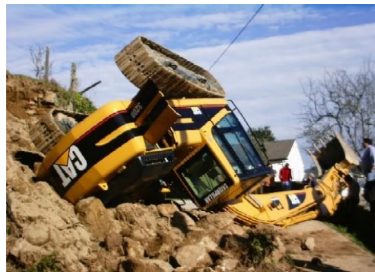
Fig. 1 Stability failure during operation of mobile working machine
