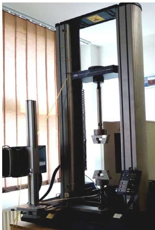
Fig.4: Instron 5560 instrument (Miskolc University)
