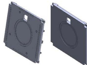
Fig. 8: Displaying the base frame before and after simplification
