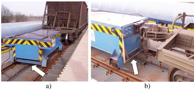
Fig.5 Attaching the ends of the ropes to the trolley
