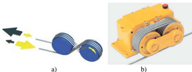
Fig.4 Friction drum with controlled placement of the rope
