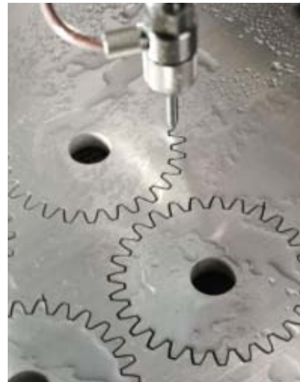
Fig. 5. Use of waterjet gear production
