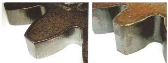
Fig. 3. Part of gearing produced by plasma arc at different thickness of gearing
