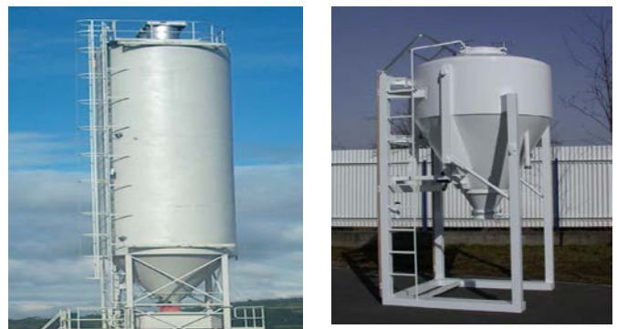
Fig.1 Two basic kinds of bulk solid storage bins
