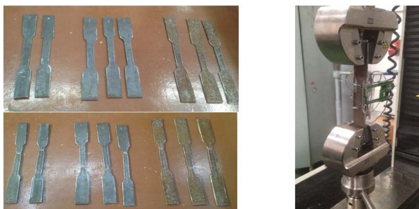
Fig.3. Coupon tests specimens and scheme of loading
